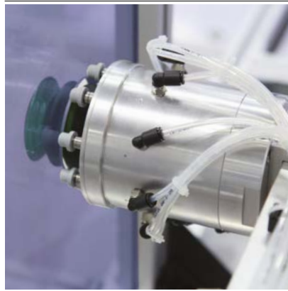
2. The positioning pins are locked at the zero position.
