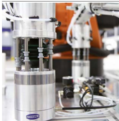
5. The gripper precisely sets up the clamping system via cup-to-cup pressure.
