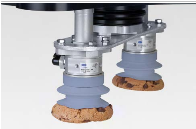
Bellow suction cups FGA of metal-detectable silicone SI-MD for handling cookies
