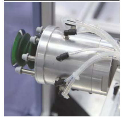
3. The positioning pins gradually move into the positions determined by the shape of the workpiece and lock in place.
