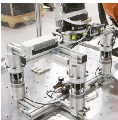
4. The gripper moves into position over the identically designed clamping system.
